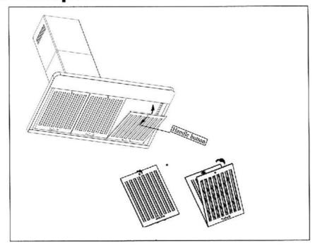
The stainless steel filters trap residue and grease from cooking.
